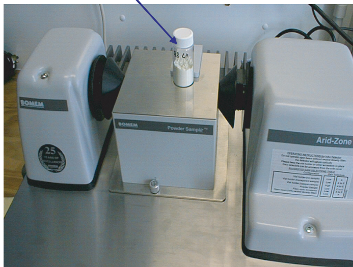
Figure 1. Photograph of the FTIR spectrometer showing the powder sampler accessory.
