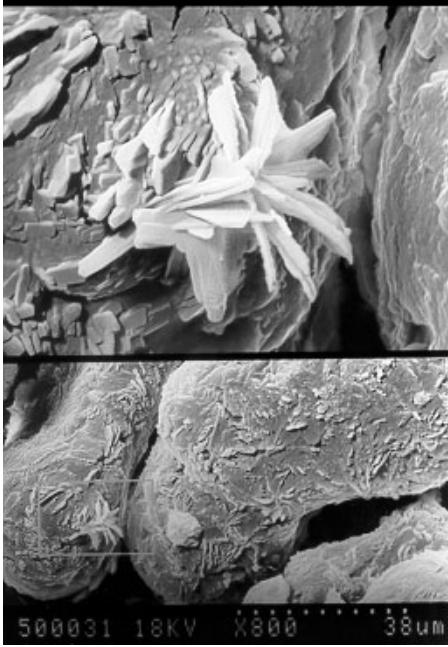
Figure 3. Electron microscopy photograph from the surface of milk powder particles after lactose crystallisation.
