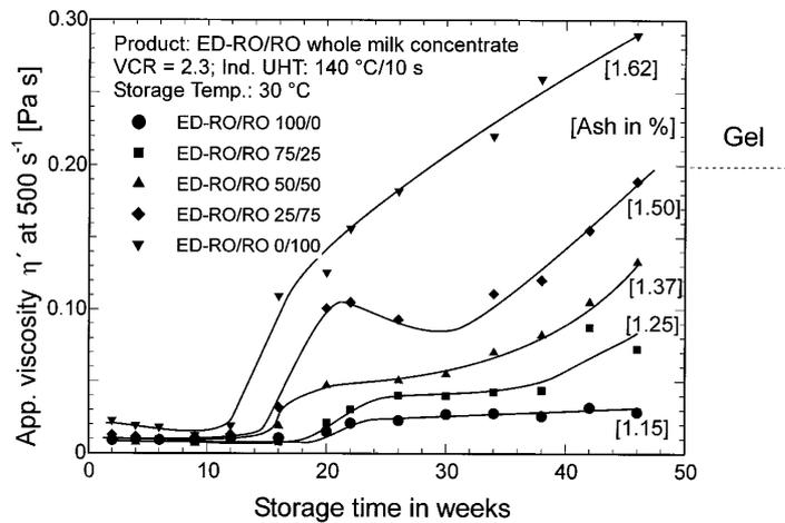
**Figure 8.** Viscosity increase during storage of the ash dependent of the milk concentrates (table inside: e.g. ED-RO/RO 25/75: 25% demineralized reverse osmosis concentrate and 75% reverse osmosis concentrate).
